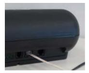
3. Connect the appropriate end of the power adapter cord into the Power socket located on the rear panel of the **SBU2000** Monitoring Unit.
