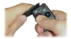
Press the red button on the Electronic Key down for one
