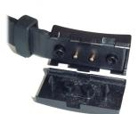
Cover the female clip with the male clip ensuring that the pins on the male clip fit correctly into the female clip (the grooves on the side of each clip must match).
