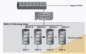
Pros: Fastest read/write performance of any of the Hybrid RAID levels High data reliability as all the data is redundant
