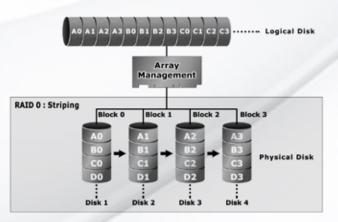
Cons: The reliability of RAID Level 0 is less than any of its member disk drives due to its lack of redundancy.
