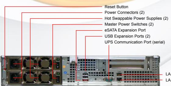
LAN 2 RJ45 Connector LAN 1 RJ45 Connector
