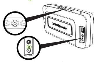
Press and hold the power button  $\circlearrowleft$  on the top of the unit for one second to turn it on.
