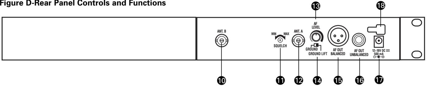
10. ANTENNA INPUT JACK: BNC-type antenna connector for Tuner "B." Attach the antenna directly, or extend it with a low-loss antenna cable. See the "Antennas" section on page 3 for more details.
