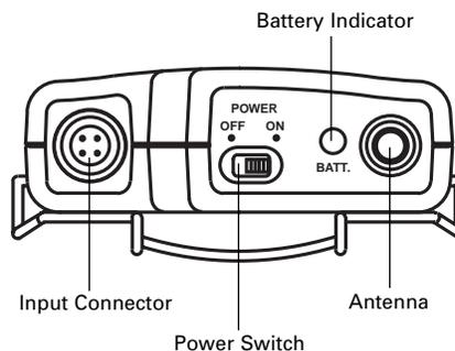
Figure H-Handheld Transmitter Bottom View
