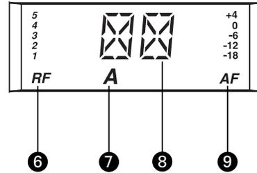
6. **RF SIGNAL LEVEL INDICATOR:** Shows the strength of the RF signal received from the transmitter.
