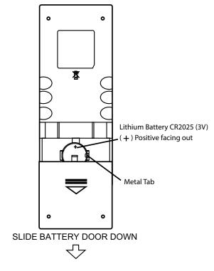
Figure 3. VX3020 Remote Control Battery Replacement.
