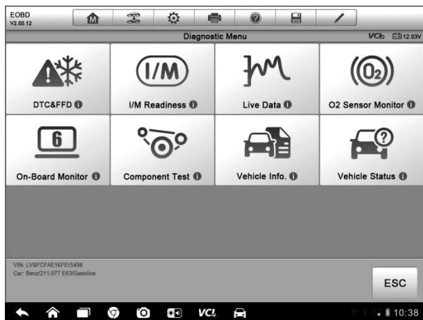
Figure 5-1 Sample OBD II Diagnostic Menu
