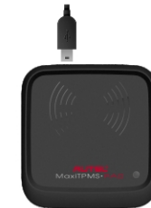
Connect Type B plug to the PAD.
