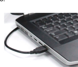
Connect Type A plug to the PC.
