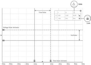
Figure 16-8 Measurement Rulers Display
