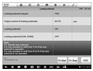
Figure 4-13 Sample Active Test Screen
