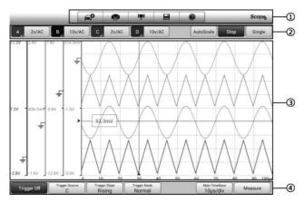
Figure 16-4 Sample MaxiScope Application Screen Layout
