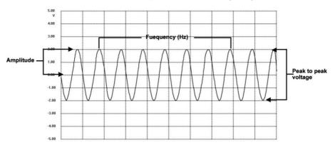
Figure 16-1 Sample Sinusoidal Waveform
