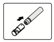
Slip the end of the accessory over the imager head and then fix the accessory.
