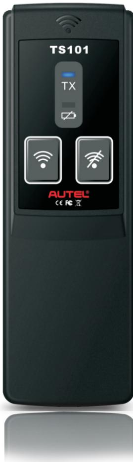
Place the TS101 90 degrees on the tire sidewall near the sensor.
