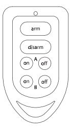
The plug 'n power Supervised Security System Cat. No 49-1000 includes a Security Console with an automatic dialer that calls neighbors or friends in the event of a break in. A battery powered RF Door/Window Sensors and battery powered RF Motion Detector to trigger the alarm, and an RF and Keychain Remote control for arming and disarming the system. All sensors and remotes incorporate random digital security coding.
