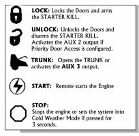
Note: Pressing the LOCK and UNLOCK buttons at the same time will activate the AUX2 output.
