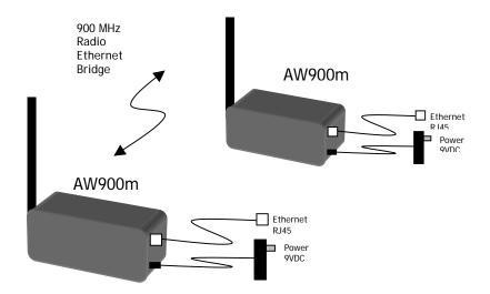
Any Ethernet device can be connected to the AW900m. The AW900m functions in place of an Ethernet cable and provides a transparent wireless point to point Ethernet cable replacement. Cross-over cables are not necessary as the AW900m automatically senses the device (client or switch.
