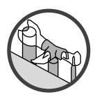
maintenance or cleaning. The pilot flame must contact the thermopile and thermocouple (see the illustration to the left). If it does not, turn the gas control valve to "OFF" and call your dealer.
