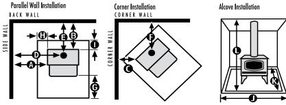
The dearances on this page are for reference only, refer to the Owner's Manual for exact specifications prior to installation.
