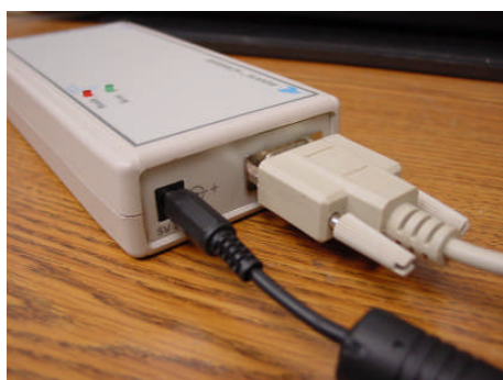
Power and serial connections to the encoder
