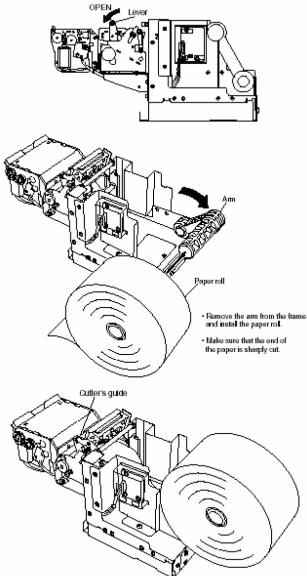
Pass the paper over the damper shaft, pass it under the thermal head, then insert the paper between cutter guides. Double check that the paper is inserted into the cutter by looking into the small wholes on the upper cutter guide. Feed the paper until the end enters the presenter's roller.
