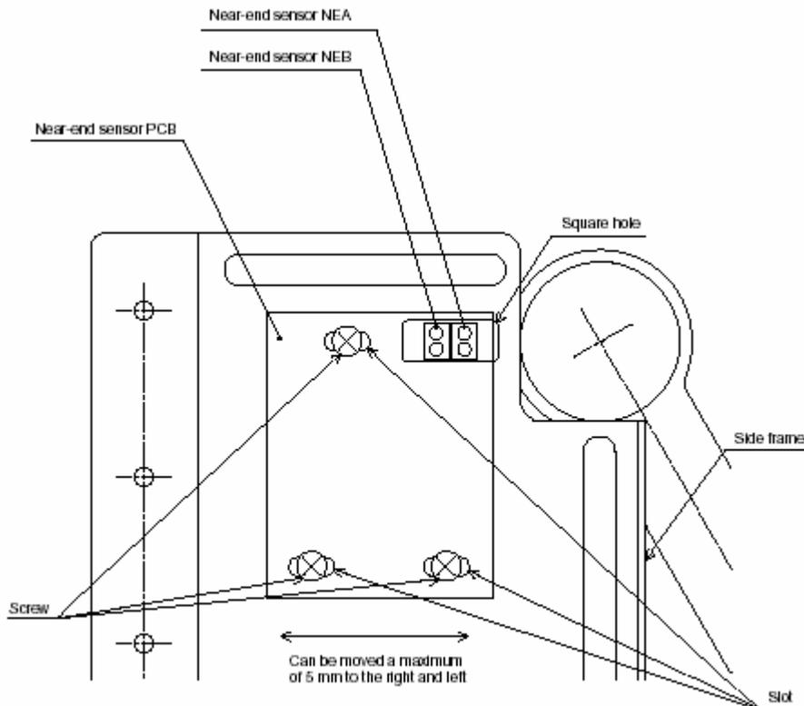
\* The near-end sensors are mounted on the back of the PCB.
