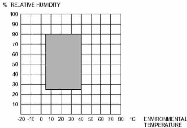
Notes- When the environmental temperature is too high, the thermal head temperature sensor is activated and the printer stops operating.
