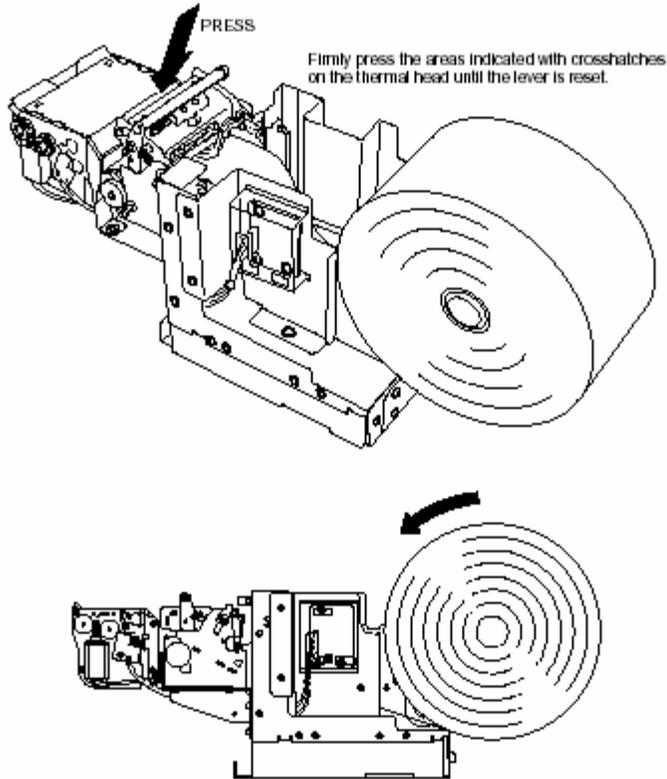
Carefully place the paper roll on the frame, then wind the roll to remove any slack in the paper.
