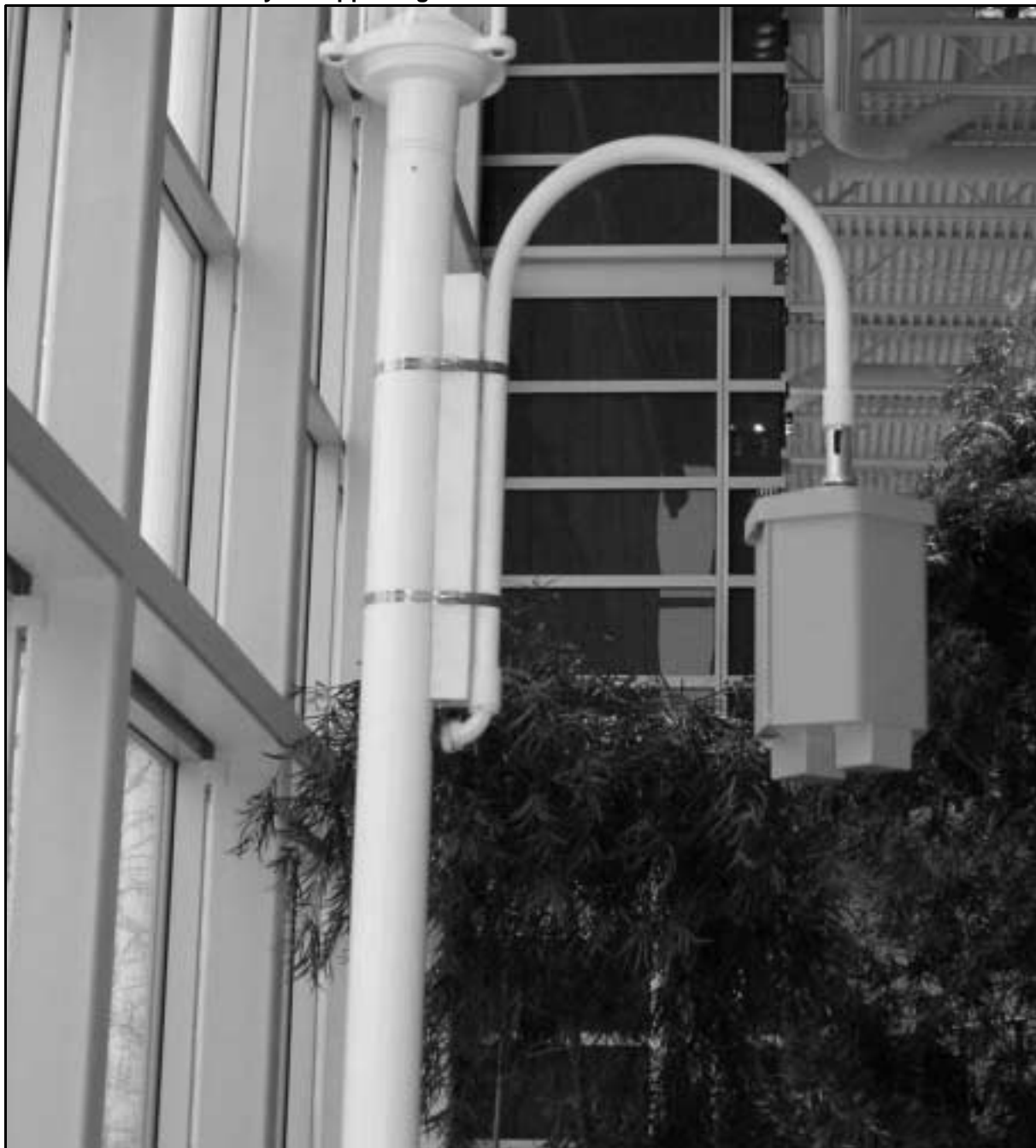
Figure 1-5 AP7220 mounted directly to supporting electrical conduit
