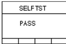
The DCSM is in stand-alone mode after the self-test. The display shows that the mobile unit is on and is ready for originating and answering calls.
