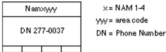
To read the ESN (Electronic Serial Number) and to access the contents of NAM1, enter a six digit security code. The factory default security code is 000000.
