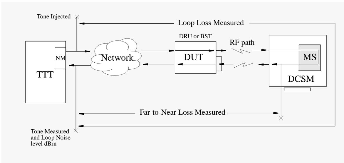
*How to Invoke the MRLT/MRHT test*
