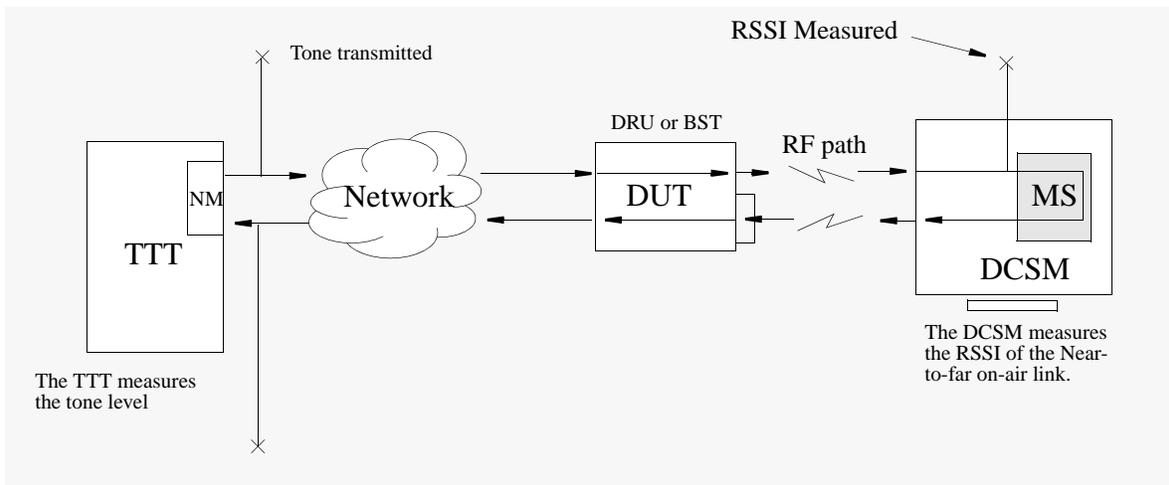
*How to invoke the MRLP test*
