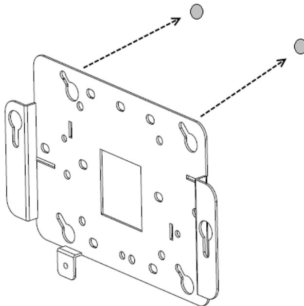
4. Tighten the screws to secure the wall mounting bracket tightly against the wall.
