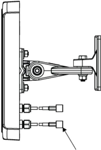
The mounting bracket is designed to use wall anchors with threaded section diameters ranging between 3.5mm and 4.5mm. If wall anchors have threaded diameters greater than 3.5mm, only the two mounting holes marked 'A' may be used. If wall anchors have threaded diameters of less than 3.5mm, the holes marked 'A' and the holes marked 'B' may be used. All wall anchors must have a head diameter of less than 10mm or the wall mounting bracket cannot be installed over them.
