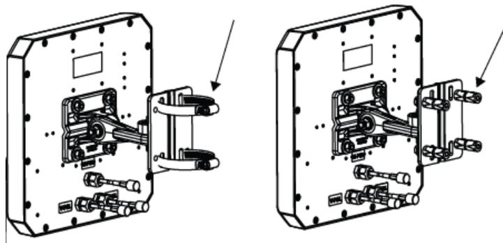
If you are installing TYCO antennas, attach mounting brackets to the wall and attach the antennas to the mounting brackets.
