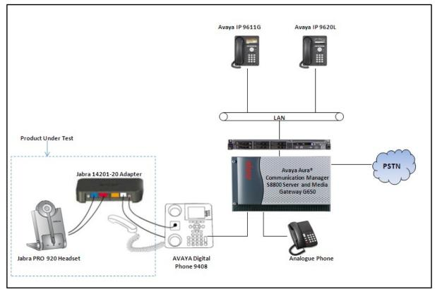
Figure 1: Reference Configuration Diagram
