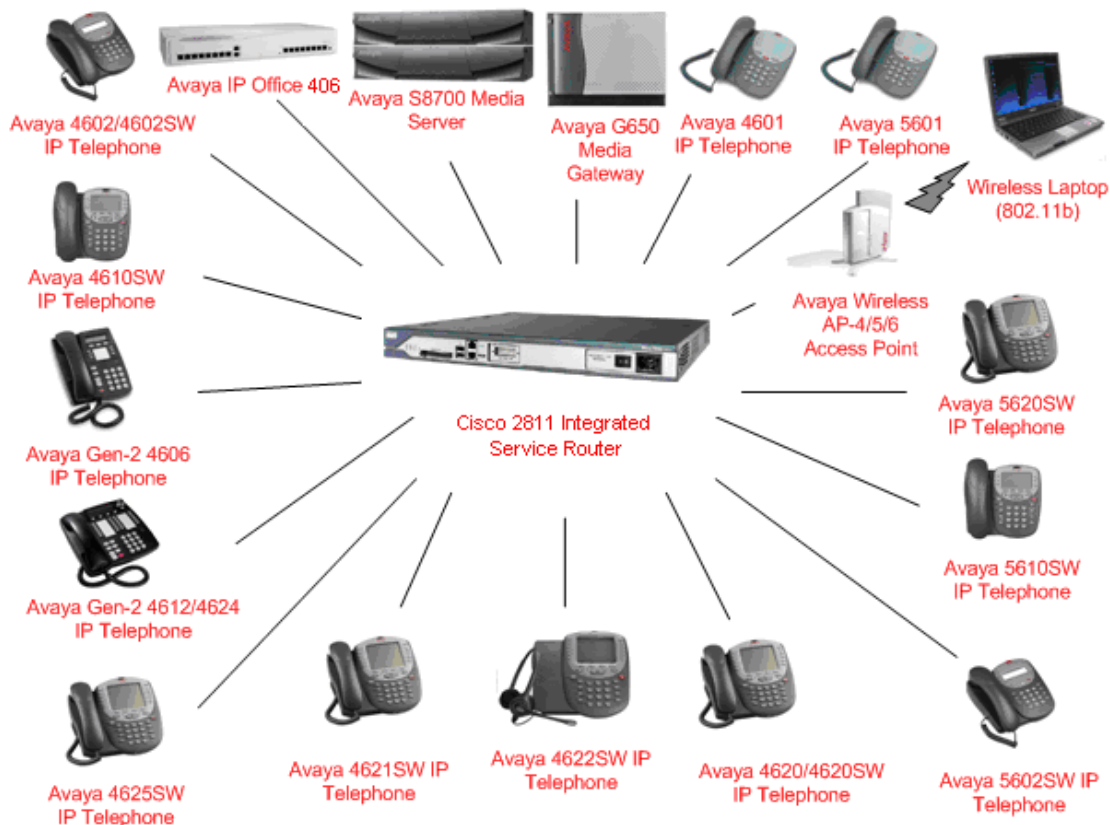
Figure 1 – Avaya 4600 and 5600 Series IP Telephones and Wireless Access Point with the Cisco 2811 Integrated Service Router
