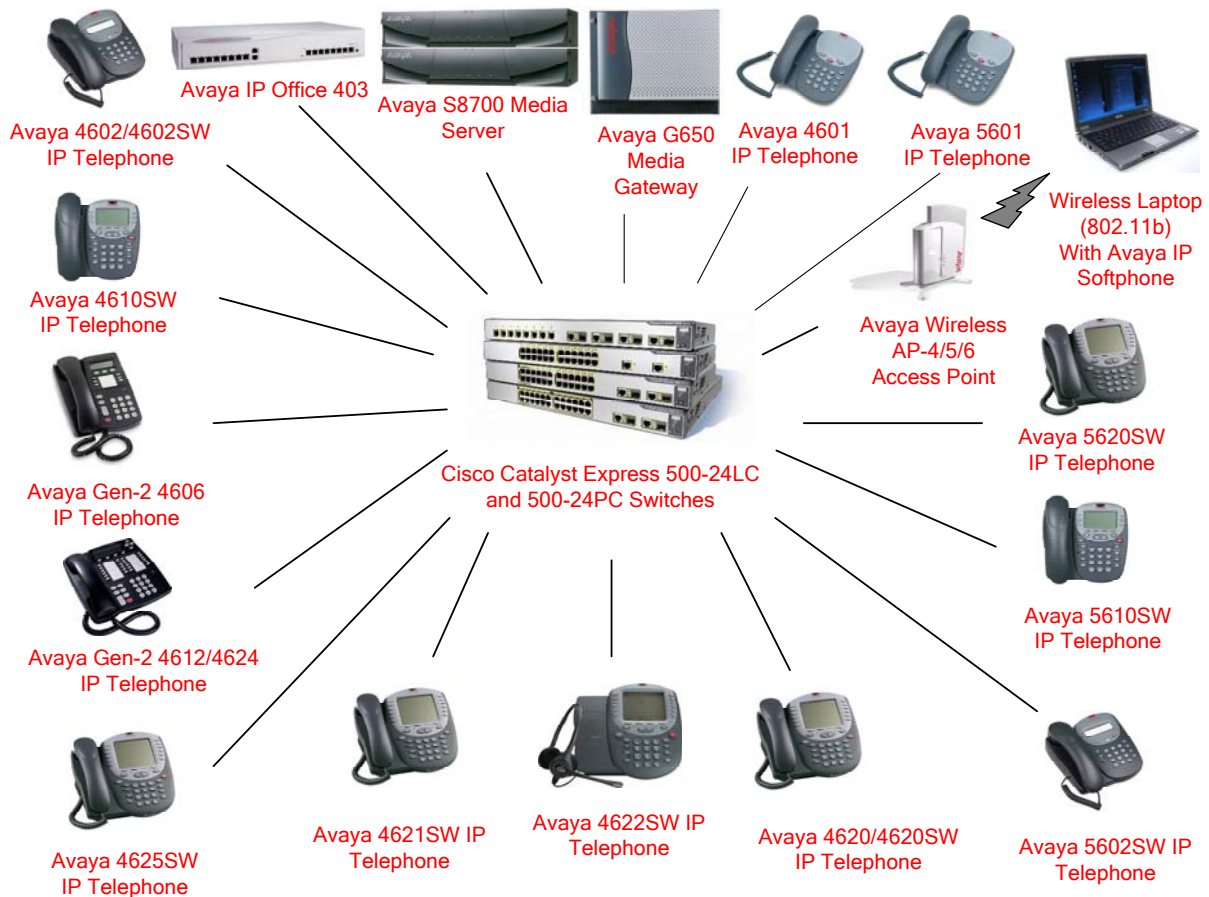
Figure 1: Avaya 4600 Series IP Telephones and a Wireless Access Point with the Cisco Catalyst Express 500-24LC and 500-24PC Switches.
