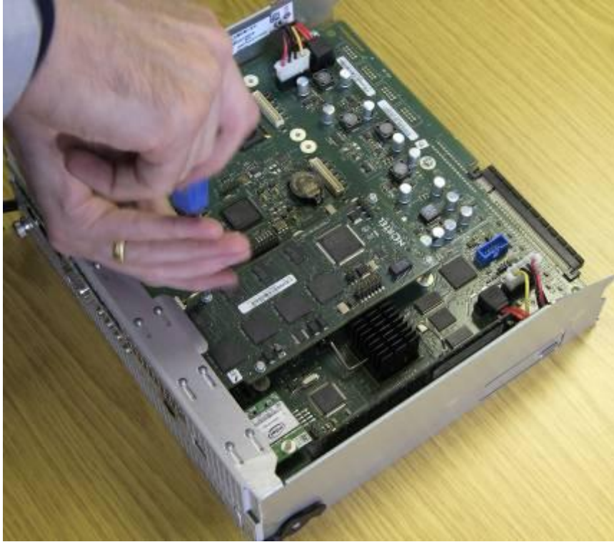
17. The Capacity Expansion Card is now secured to the Base Function Tray.
