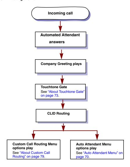
If an incoming call has a CLID value that matches an entry in the CLID Routing Table, the call is directed according to the CLID Routing Table rather than the Greeting Table. After the call is directed, the call disconnects or returns to the routing according to the Return to Auto-Attendant setting. For more information about the Return to Auto-Attendant setting, refer to "Setting the Auto Attendant properties" on page 71.
