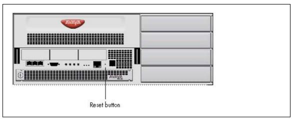
The figure Reset switch location on BCM50 on page 37 shows the location of the reset switch on the BCM50.
