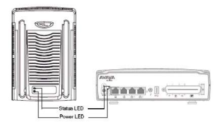
The LED states with descriptions of LED combinations table describes the meaning of the system status LEDs after the system turn on and is in service.
