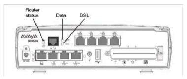
Figure 4 ADSL router LEDs on the Avaya BCM50a and Avaya BCM50ba main units (BCM50a shown)
