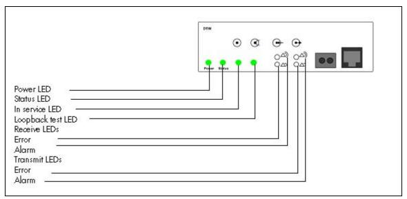
The DTM LED functions table describes the functions of the DTM LEDs.
