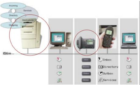
The i2004 Internet Telephone and the Terminal Proxy Server (TPS) software are built on H.323 standards established by the International Telecommunications Union for multimedia communications over packet-based networks such as a corporate LAN. This means your phone will work in harmony with other IP-based software and hardware.
