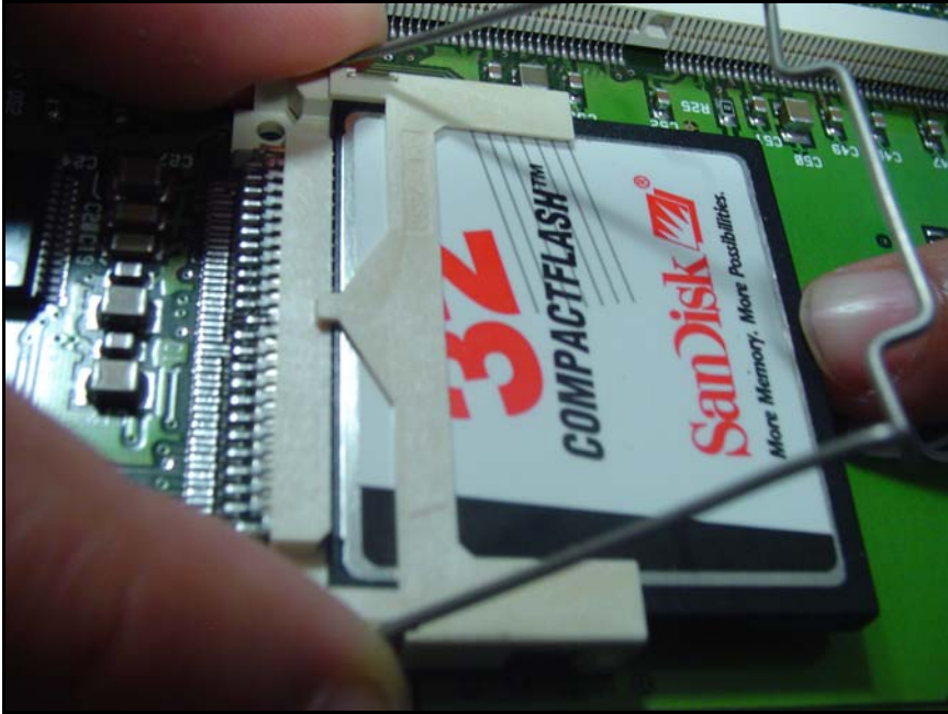
Figure 63 Seat CompactFlash card
