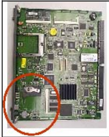
Figure 60 CompactFlash card socket on Media Card
