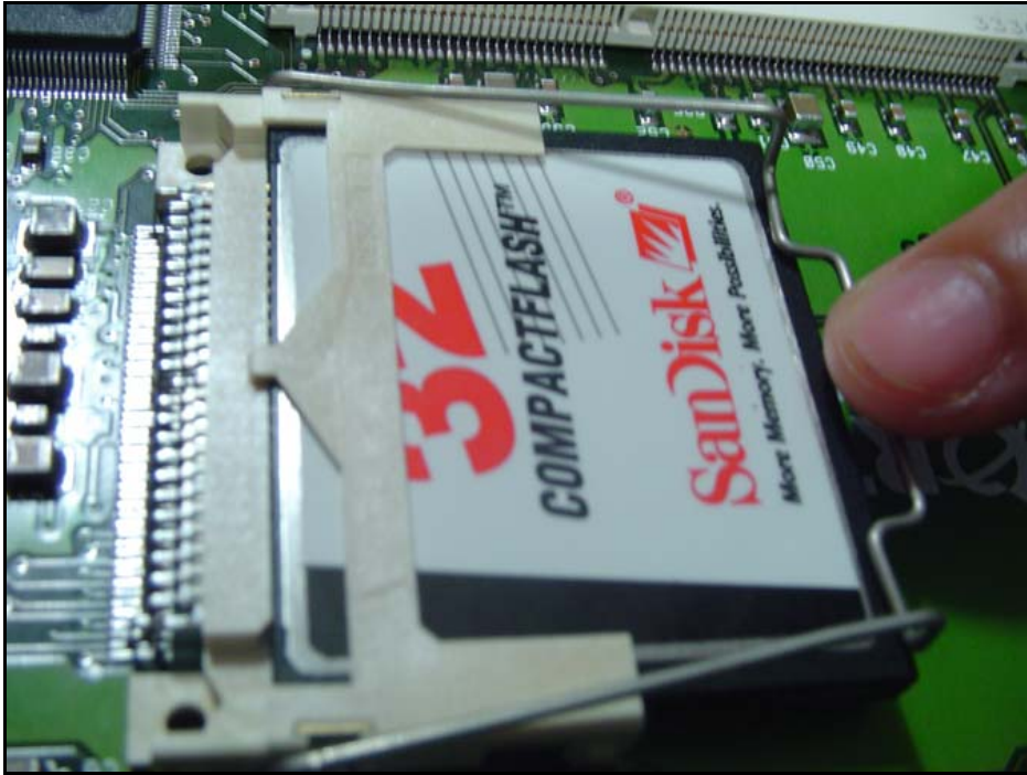
Figure 64 Lock card into place
