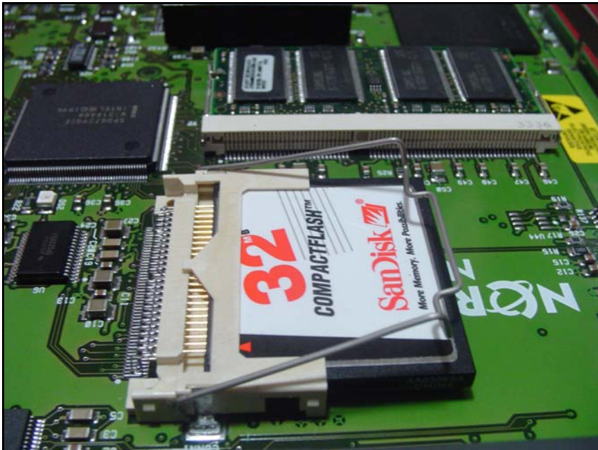
Figure 238 Lift the metal clip on the CompactFlash card
