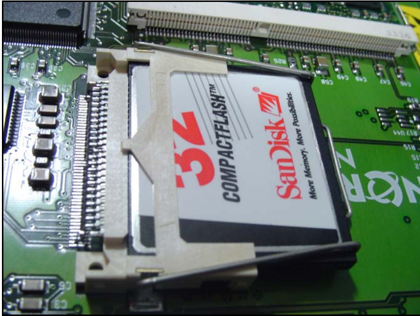
Figure 65 CompactFlash card locked into position
