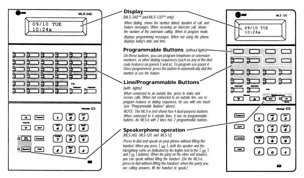
Intercom Buttons. Press either button to place an inside (intercom) call to another extension. Volume Control Buttons. Press to decrease (▼) or increase (▲) the volume of the ringer, speaker, and handled:
