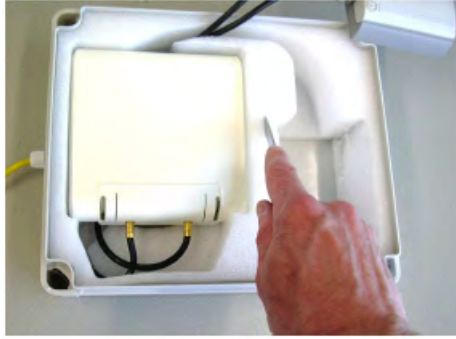
Figure 83: Cutting the foam to allow the antenna to fit into it, in the required position
