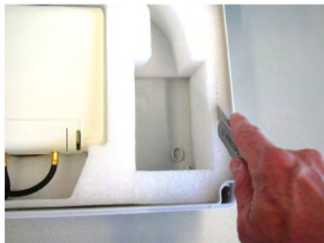
Figure 82: Cutting the foam to allow the antenna to fit into it, in the required position
