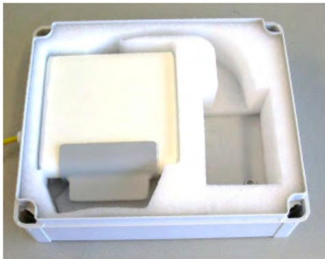
Figure 68: 4720 DAP in position in the cabinet
