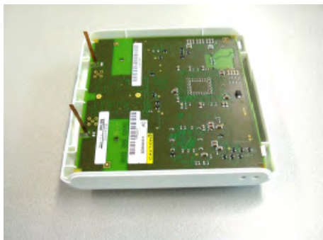
Figure 43: Bend Antennas carefully into vertical position
