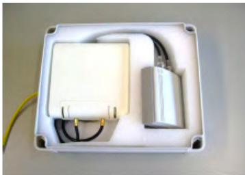
Figure 81: Antenna does not fit into the hole
