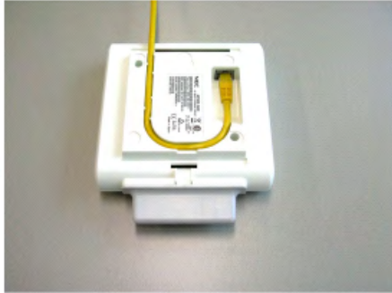
Figure 49: Cable at rear side of the cabinet
