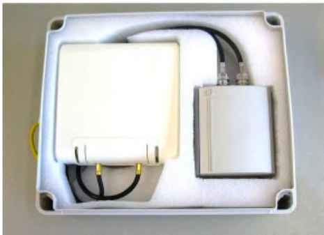
Figure 84: 4720 DAP and directional antenna in their positions
