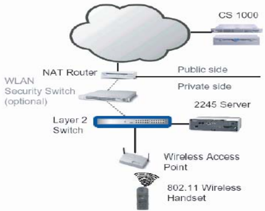
Figure 5 NAT network configuration 2 – with a security switch
