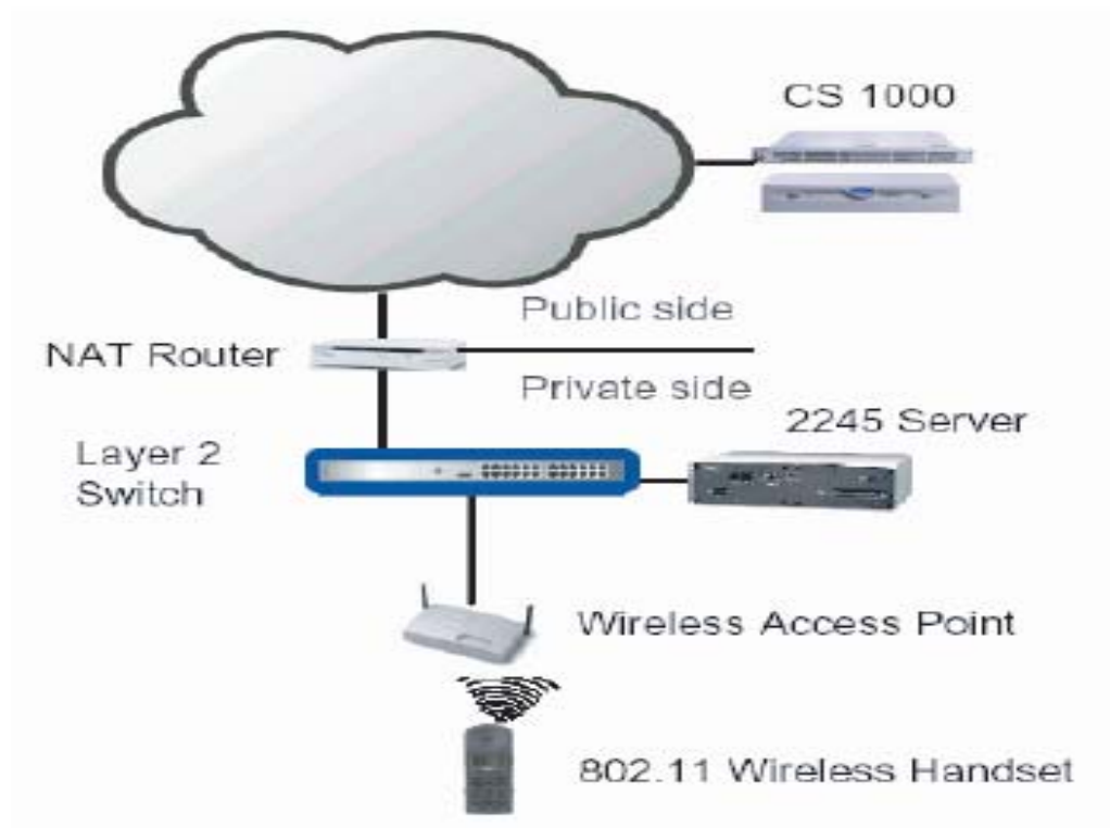
Figure 4 NAT network configuration 1 – without a security switch
