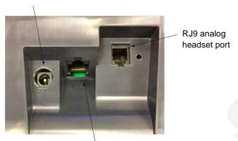
RJ45 10/100/1000 Mbps Gigabit Power over Ethernet port
