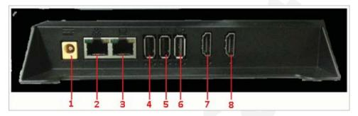
Number Name Power connector RJ45 Gigabit Ethernet PoE connector 2 3 RJ45 Ethernet personal computer connector 4 USB 2.0 connector 5 USB 2.0 high-power gadget charging connector. As the port uses only the spare power, the charging speed may vary based on whether power supply is through AC, PoE, or SP-PoE. 6 USB camera connector 7 Digital video display out connector 8 Digital video display in connector
