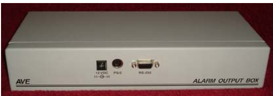
Figure : AL-16 RS-232 & Power Connector
