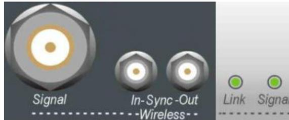
**Figure 9: System - AN-100U/UX Front Panel Wireless Section**
