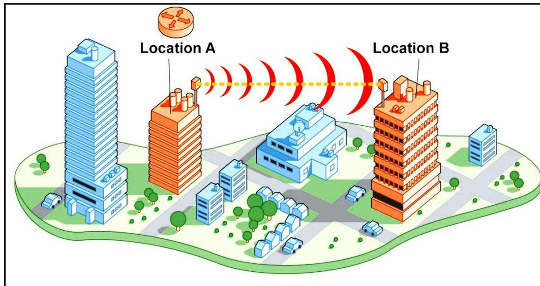
**Figure 4: System - PTP Line of Sight Deployment**
