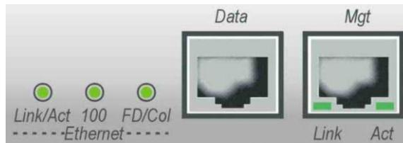
**Figure 10: System - AN-100U/UX Front Panel Ethernet LEDs and Ports**
