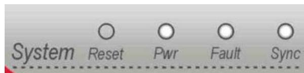
**Figure 6: Front Panel: Reset Switch and System LEDs**
