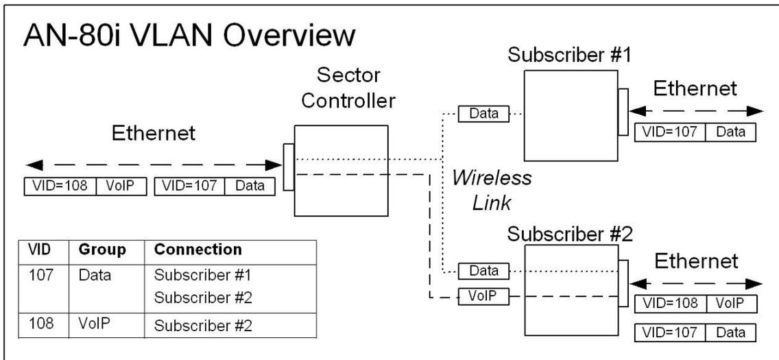
Figure 24: PMP - VLAN Tagged Traffic Example
