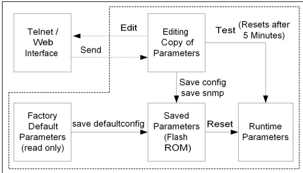
Figure 39: Diag: - Saving Parameters in NVRAM
