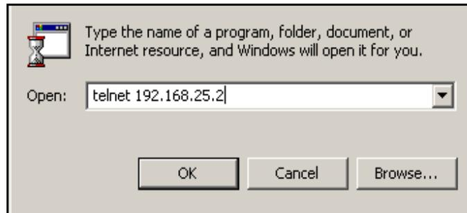
**Figure 37: CLI - Connecting via Telnet**
