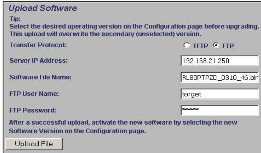
Figure 16: Web - Upload Software Screen
