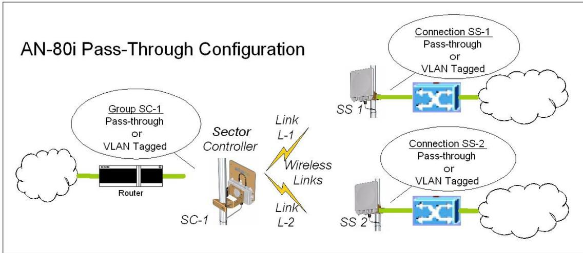
Figure 23: PMP - Basic Pass-through Group Configuration
