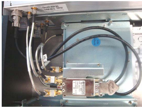
Figure 5-2. IRU 600v2 Tx Switch and RFUv2 Connections
