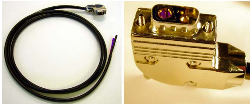
Figure 6-4. Power Cable and Connector
