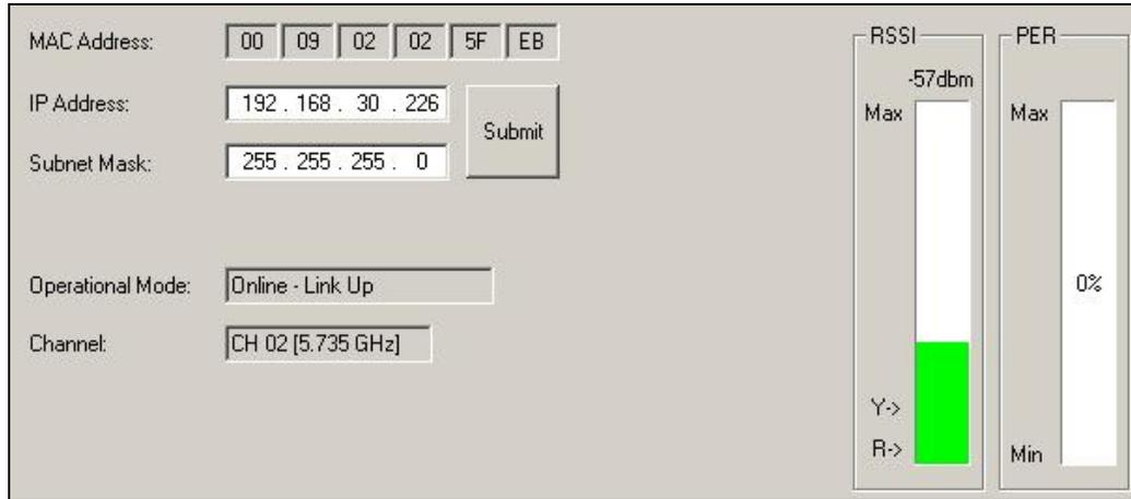
Figure 13: Link Mgr - Basic Installation Screen - Master
