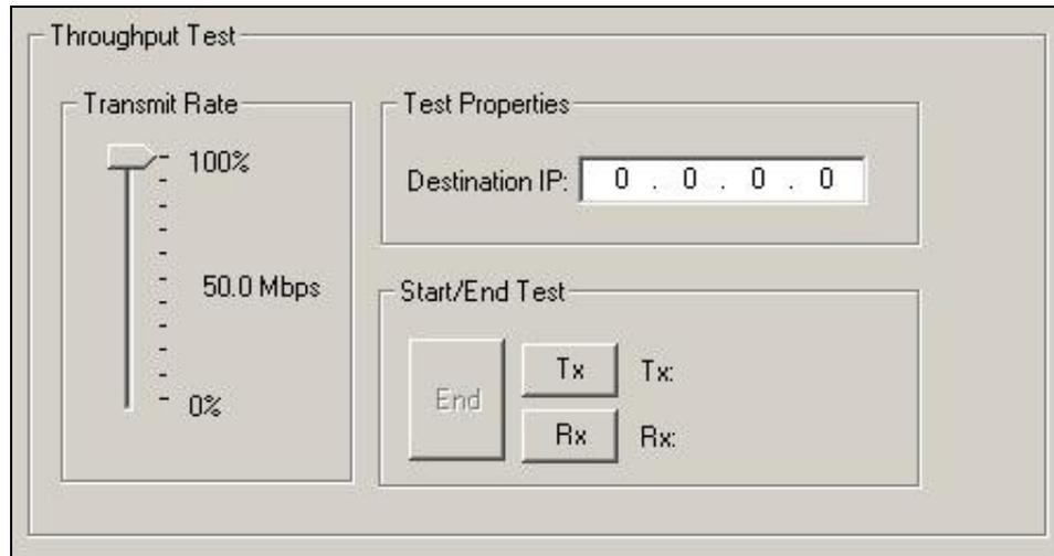
**Figure 24: Link Mgr - Tests Screen - Throughput test**
