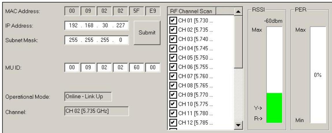
Figure 14: Link Mgr - Basic Installation Screen - Slave
