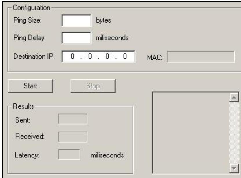
**Figure 25: Link Mgr - Tests Screen - Ping Test**
