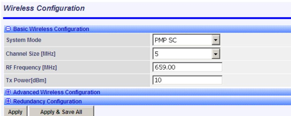
**Fig. 3: Web - Wireless Configuration Screen -- Sector Controller**
