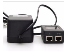
c) Power over Ethernet Injector (PHIHONG PSA 16U-480)
