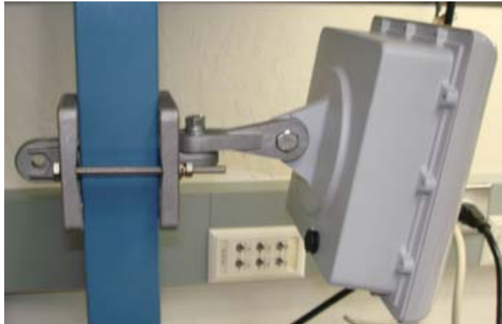
Figure 2-2. Subscriber Station mounting assembly
