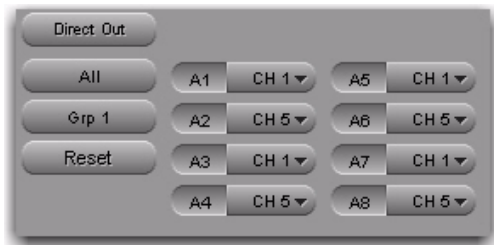
Channel pop-up menus alternating top to bottom between channels 1 (CH1) and 5 (CH5)
