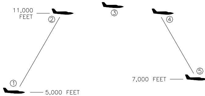
Figure 6 Example of Altitude Alerter Operation
