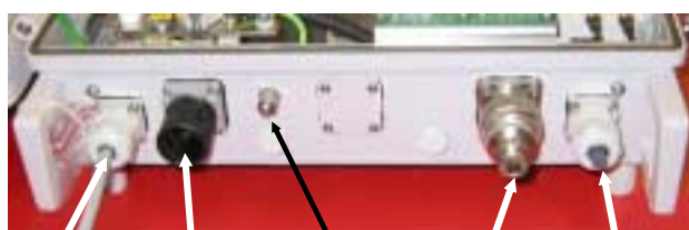
Power Fiber cable input Ground Server antenna External alarms
