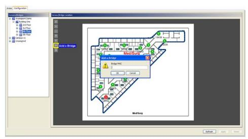
Figure 50 - Placing Awarepoint Bridge Using B Button
