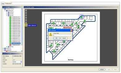
Figure 55 - Placing Awarepoint Sensors using S button
