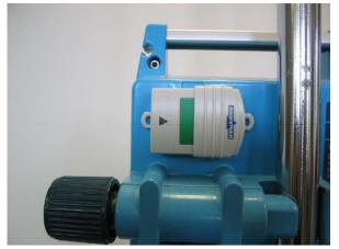
Figure 64 - Tag Double-Sided Tape Attachment
