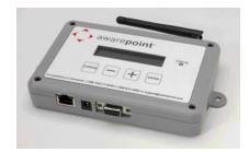
**Note**: Do not configure the B2 Bridge using the serial cable connection. If a serial cable is connected to a Bridge, it will place the Bridge into a stalled state and will need to be sent back to Awarepoint via RMA.
