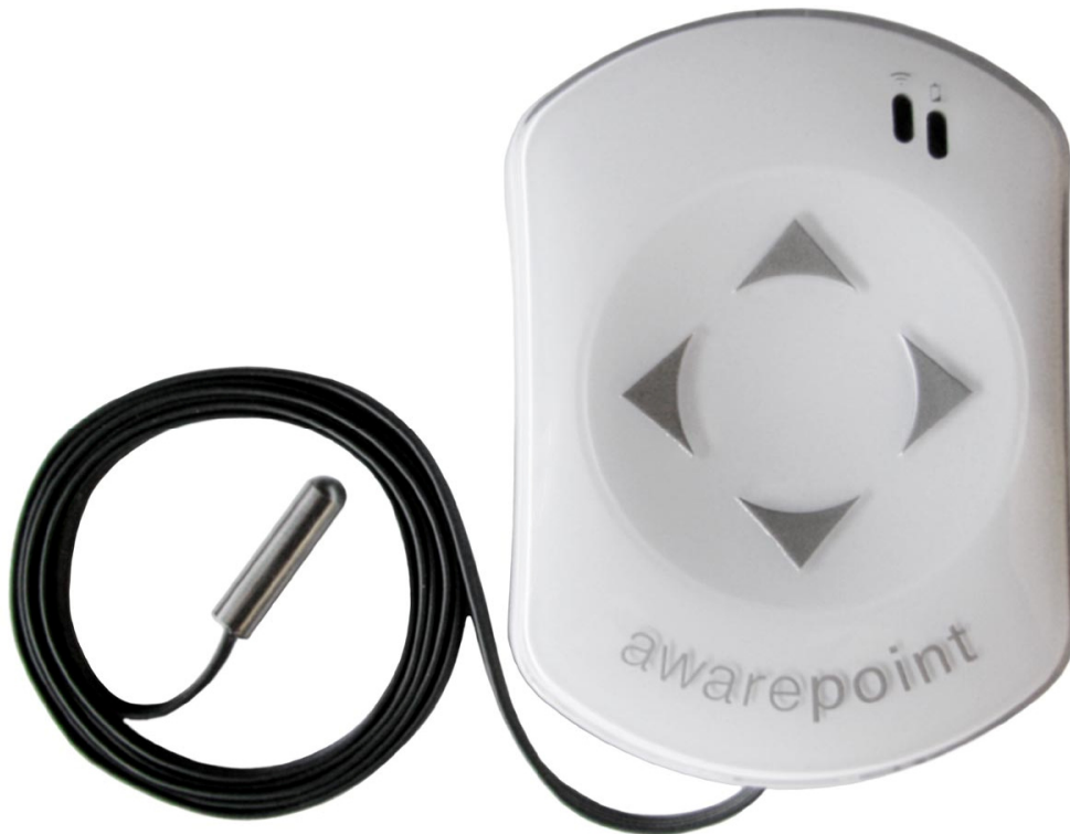
Figure 2: Tag, with temperature probe
