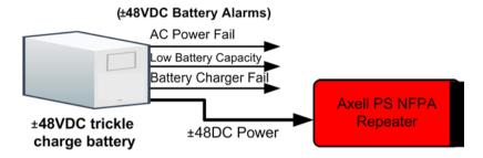
Figure 3-8. NFPA Battery Power Connections
