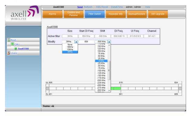
The selected deviation will be added to the positioning of the filter. For example, if you select **250 KHz** shift for the **865 MHz start frequency**, the DL and UL frequencies will be displayed as follows: **DL Freq. range: 864.75 MHz-867.75 MHz**
