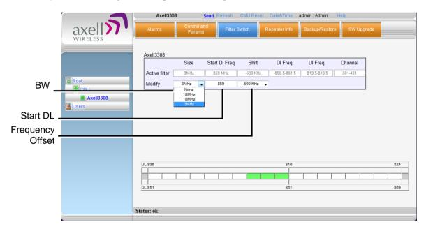
In the example below the selected BW is 3MHz and the DL start frequency is 859MHz.
