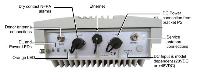
Figure 1-2. BSR 3308 BSR PS NFPA Front Panel Interfaces
