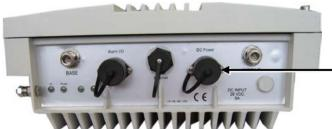
\_DC Input connection from system AC/DC Converter
