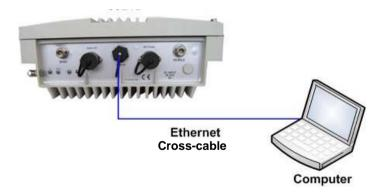
Figure 4-1. Local Ethernet Cross-cable Connection
