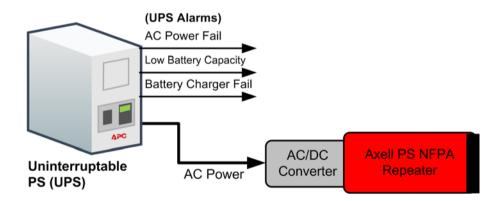
Figure 3-7. NFPA UPS Power Connections
