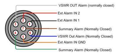
Figure 3-9. Alarm Connector Pinout
