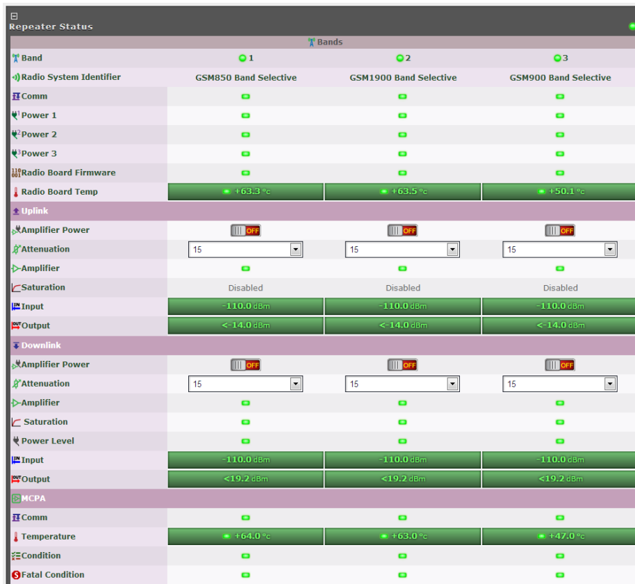
Figure 5-3. MBF-40 Repeater Status
