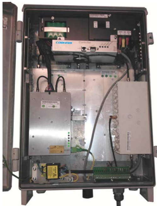
Figure 2-15. Example of Open Repeater Model
