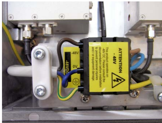
Figure 3-35: -48VDC Power Connections
