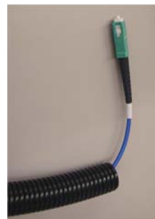
Figure 3-25: Run Optic Fibers through Sleeve
